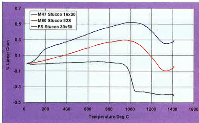
Figure 3. Thermal expansion of fused silica slurry with fused silica, Mulgrain 47, and Mulgrain 60 stucco.
