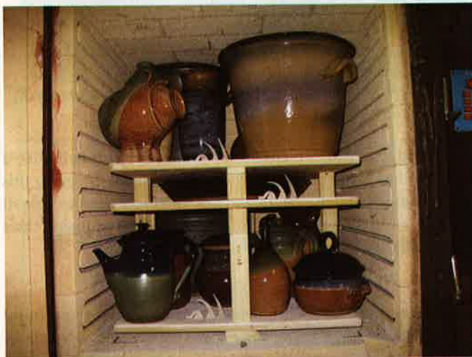
Figure 2. Cones placed inside the ware setting allow you to verify that the desired heatwork has been achieved.
