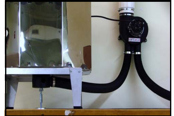
Typical wall mounted installation with 2 kilns
