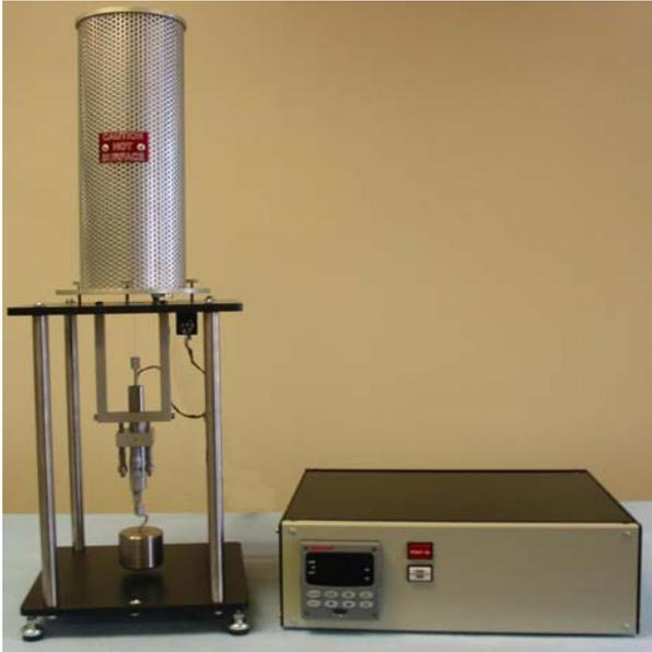
**Automatic Annealing & Strain Point results in less than 25 minutes.**
