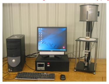
The annealing and strain points of a glass are widely used production control parameters. Changes in the annealing and strain point temperatures are indications of chemistry changes.
